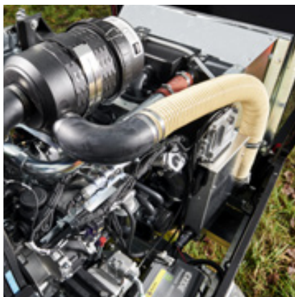
Motor Hatz 4H50 de 55,0 kW
