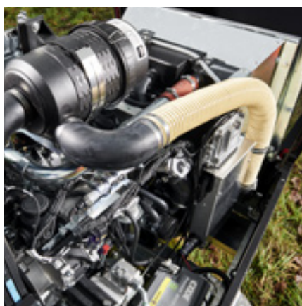
Hatz 4H50 engine with 55 kW
