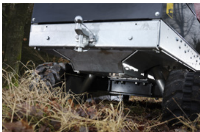
Ground clearance of 250 mm, easy service and reinforced hose protection.
