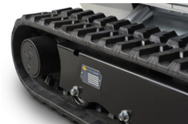
Ground clearance of 215 mm. Easy service and solid protection of hydraulic hoses.
