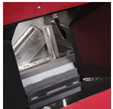
Aggressive horizontal rollers with 8.5" roller opening (216x265 mm)
