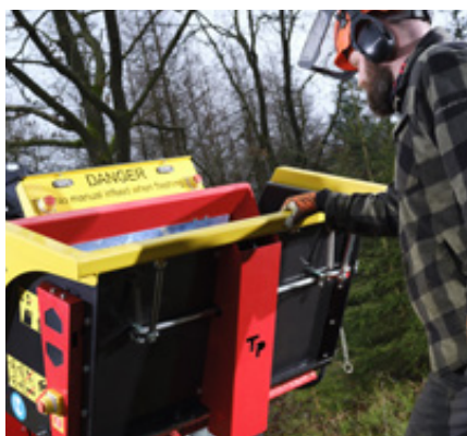
Easy handling of the reinforced heavy-duty funnel thanks to gas spring
