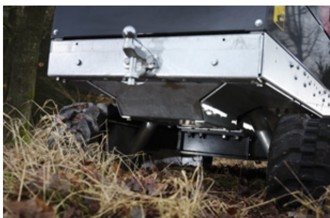
Ground clearance of 250 mm, easy service and reinforced hose protection. Variable track width.
