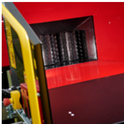
Vertical infeed rollers from TP forest design
