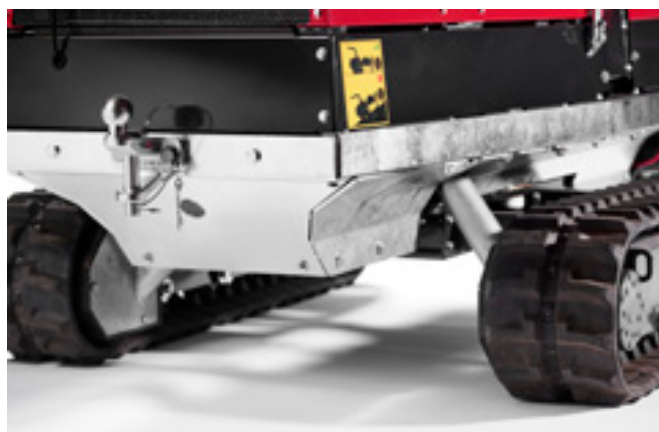
Ground clearance of 8", easy service and reinforced hose protection. Variable track width 45-53"
